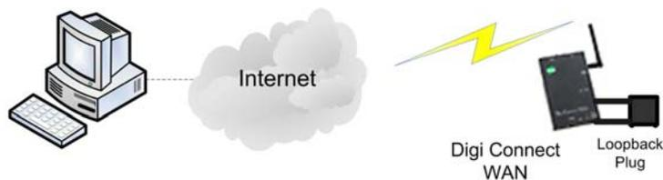
Standard Cellular to Serial Test setup
