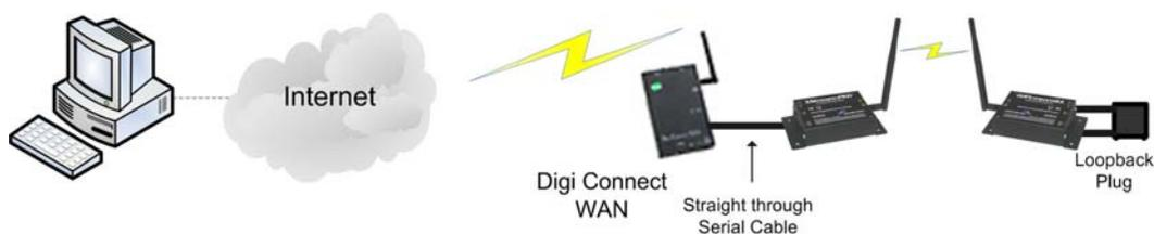
Cellular to Serial Test setup with radios
