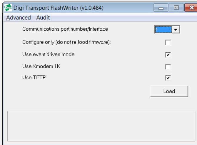
Select the communications port number (on your PC) that you connected the RS232 cable to.
