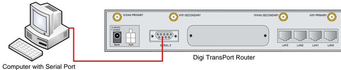
Connect the ASY 0 or Serial 0 port of the Digi TransPort router to the Serial Port of the computer. The serial cable used should be straight thru. Please refer to the following document for serial ports pinouts: [http://ftp1.digi.com/support/documentation/Transport\\_Serial\\_Pinouts\\_rev\\_3.pdf](http://ftp1.digi.com/support/documentation/Transport_Serial_Pinouts_rev_3.pdf)
