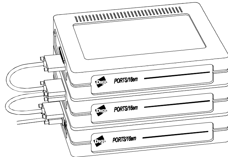
Figure 30. Three PORTS/16em modules cabled together
