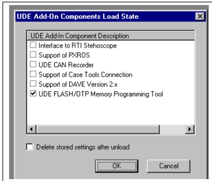
Save the workspace and open the Flash Programming tool, to enable the internal Flash support. Setup the programming tool:
