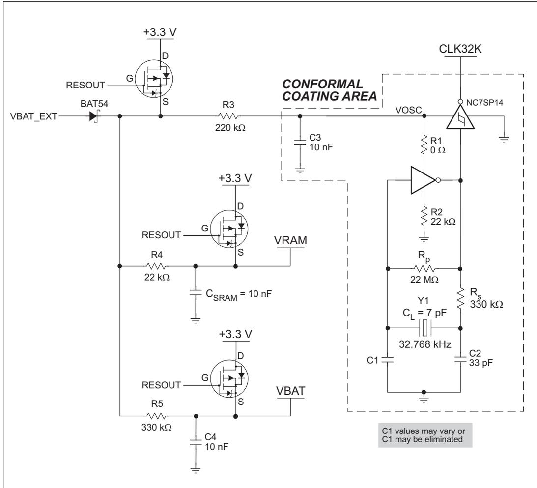
**Figure 6. Alternative Low-Power Circuit for Rabbit-3000A-Based Systems**
