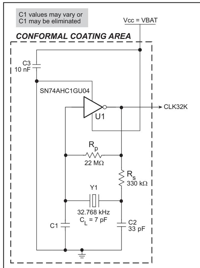
**Figure 5. 32.768 kHz Circuit for Applications not Battery-Backed**
