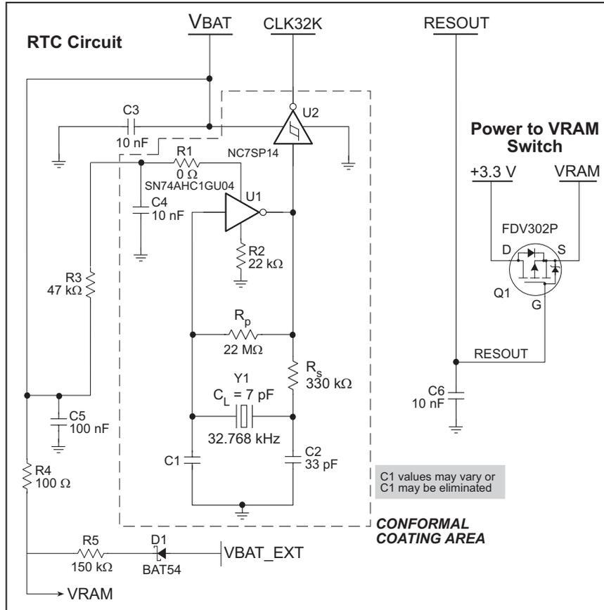
**Figure 4. 32.768 kHz Oscillator and Battery-Backup Circuit for Rabbit-3000-Based Systems**
