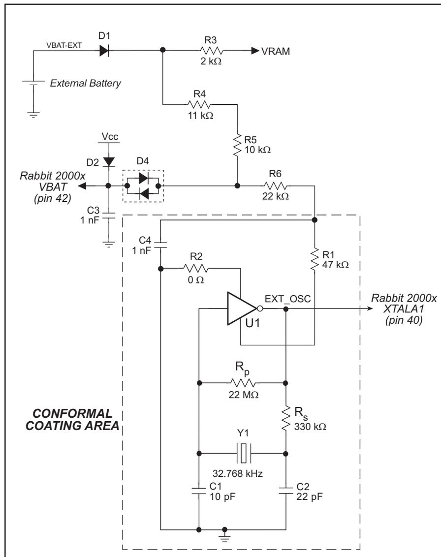
**Figure 2. Rabbit 2000x 32.768 kHz Oscillator and Battery-Backup Circuits**
