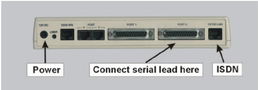
The above picture is the rear panel of an IR2140 Router. Other types of unit, such as the IR2110 and GR2130 routers may have slightly different back panel layouts, however, ISDN BRI, 12V DC and PORT 0 will still be clearly marked as above.
