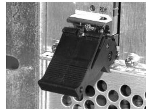
Figure 1. Ejector Handle in Unlocked Position
