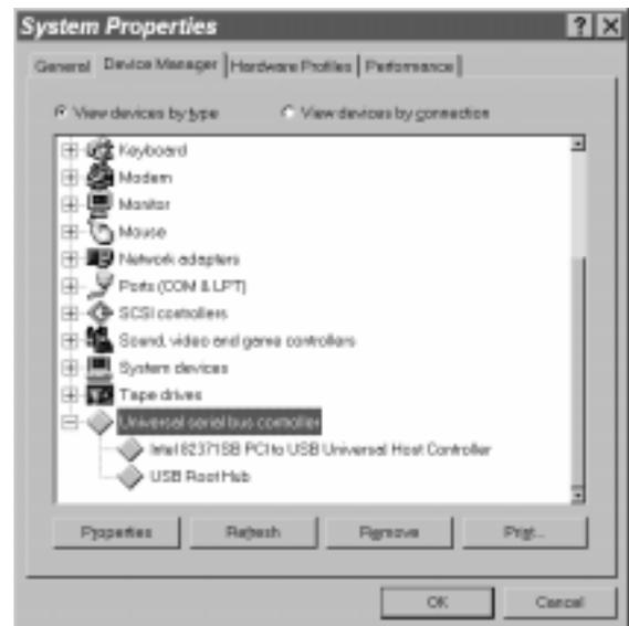
Figure 2: Example of the USB Devices Listed in the Device Manager Tab
