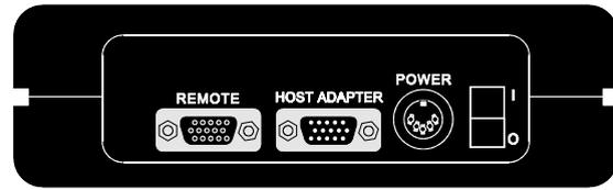
Figure 39. Side Panel of C/CON-8 or C/CON-16 module
