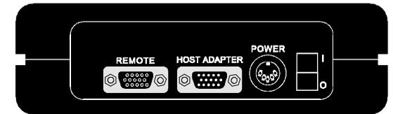
Figure 36. Side Panel of C/CON desktop concentrator
