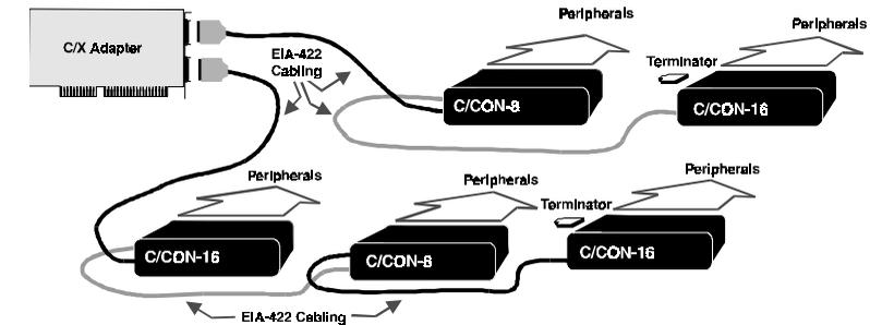
Figure 34. Example C/X setup (desktop concentrators)
