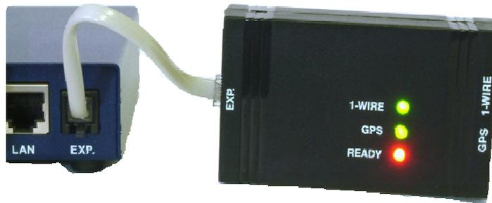
Figure 1 1 Wire Telemetry POD
