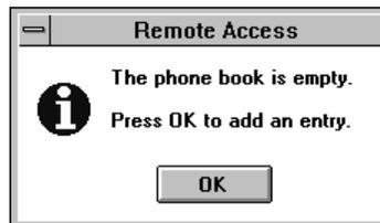
If the Remote Access phone book already has entries in it (i.e. you have installed RAS prior to the installation of the Digi ISDN adapter card and have added entries to the phone book for use with other installed communications ports), launching Remote Access opens the Remote Access window directly (without prompting for you to add an entry).
