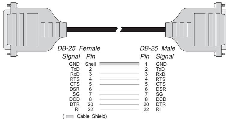
To connect a DB-25 equipped Xr board to a modem, use a standard “straight-through” cable (see Figure 3) to connect the modem to one of the DB-25 connectors on the fan out cable or connector box.
