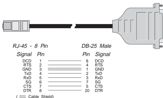
If you wish to build an 8-wire modem cable for an RJ-45 equipped board, use an 8-pin RJ-45 plug wired as shown in Figure 6.
