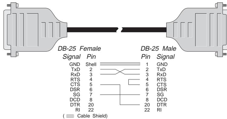
Most terminals and printers use Data Terminal Ready (DTR) for Ready/Busy hardware handshaking. The cable shown in Figure 8 supports this method.
