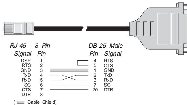
Most terminals and printers use Data Terminal Ready (DTR) for Ready/Busy hardware handshaking. The cable shown in Figure 12 supports this method.
