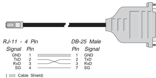
The cable shown is a three-wire null modem cable—that is, Transmitted Data on one end of the cable is connected to Received Data at the other end, and vice versa.
