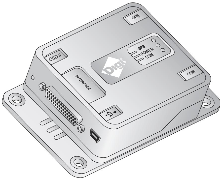
The Digi X-Trak 3 device delivers a powerful yet cost effective asset management solution by combining a programmable telematics device with an easy-to-use development environment and iDigi management platform. The Digi X-Trak 3 can be programmed using open source Python or the iDigi Device Integration Application (iDigi® Dia). Digi also provides application developers with a familiar Eclipse-based Integrated Development Environment for rapid application development.
