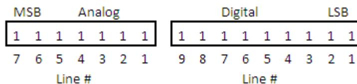
The number of analog samples is dependent on the mask. If none of the Analog mask bits are enabled, the 2-byte analog samples will not be present within the byte structure.
