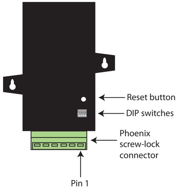
The adapter is switch-selectable between RS-422 half duplex, RS-422 full duplex, and RS-485 modes (see DIP switches, below). The function for several pins varies between RS-422 and RS-485 modes.
