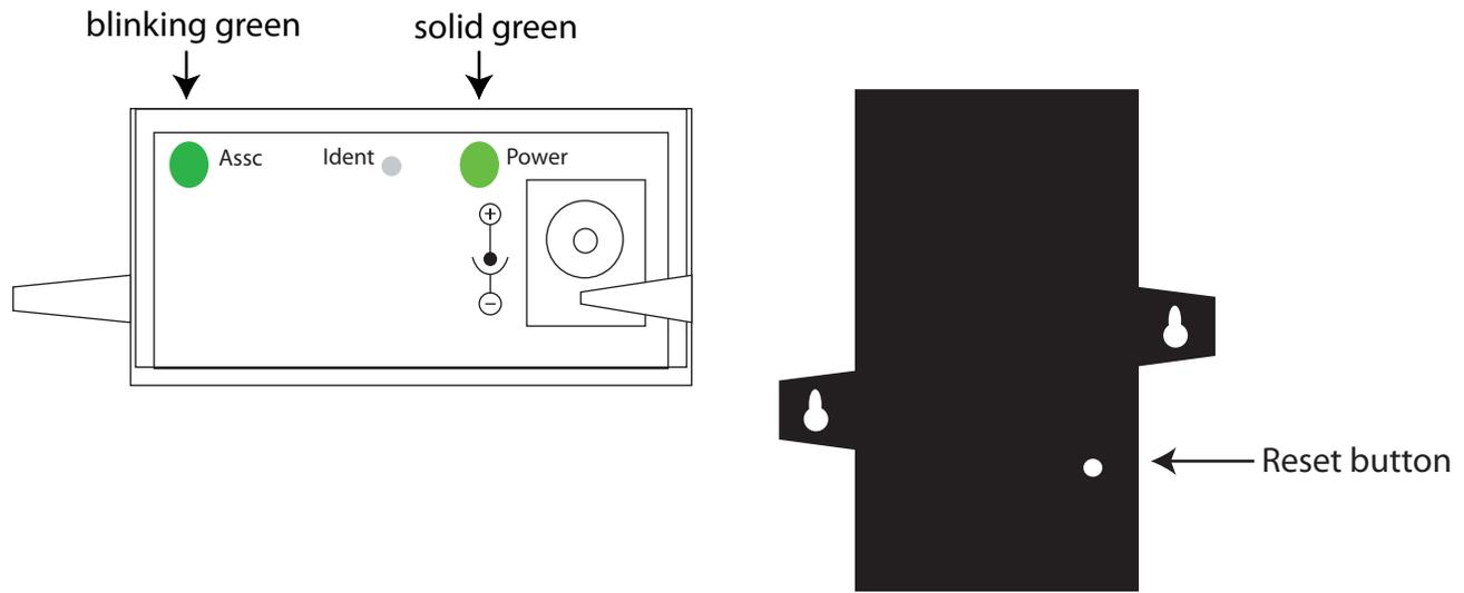
**Power LED:** Indicates that power is on. Illuminated only when adapter is connected to external power only, not when powered by batteries. Not available in lithium-battery models.
