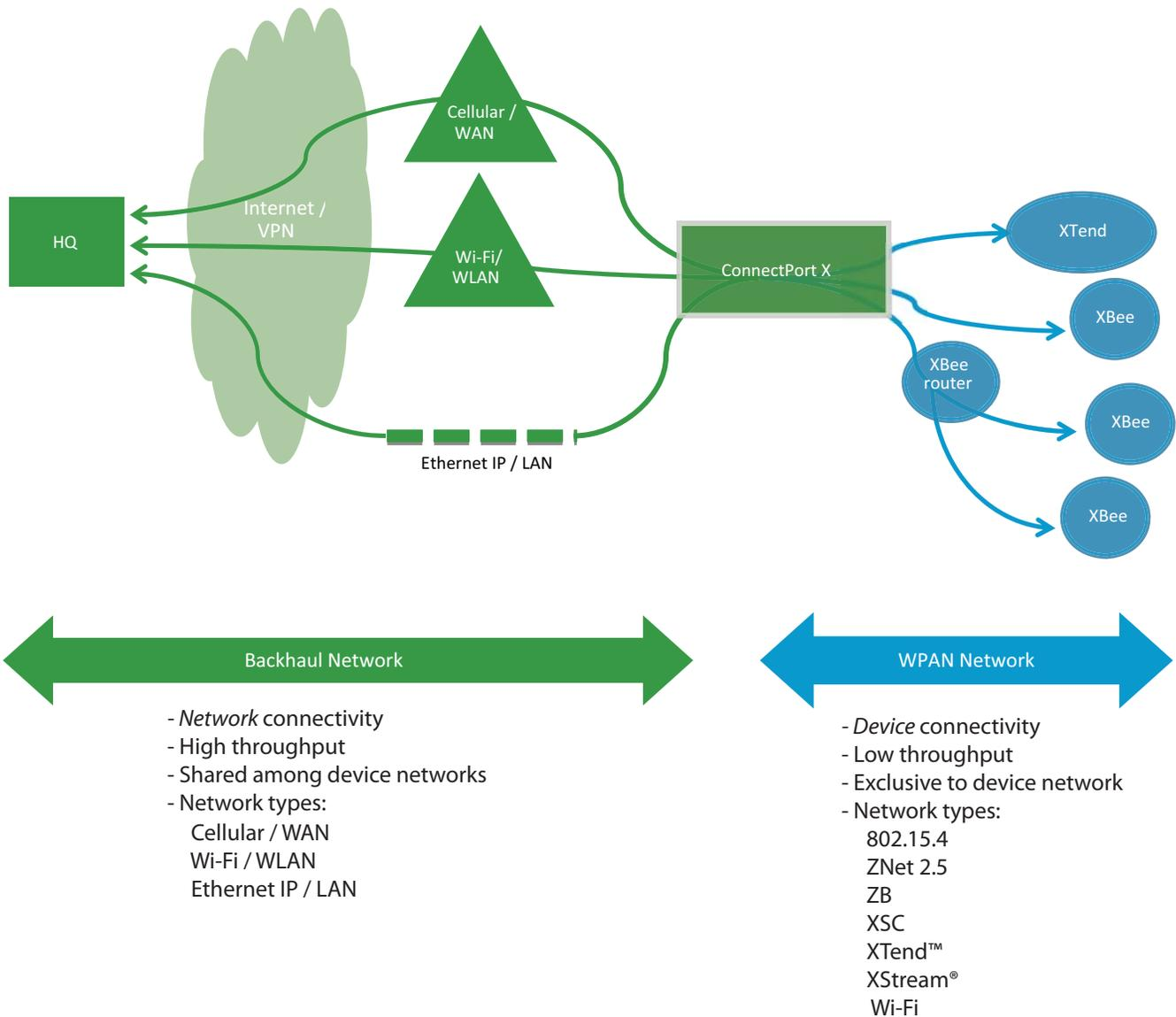
**Drop-in Networking:** Involves *end-to-end device-to-network connectivity*, commonly through gateways, routers, adapters, and embedded modules.
