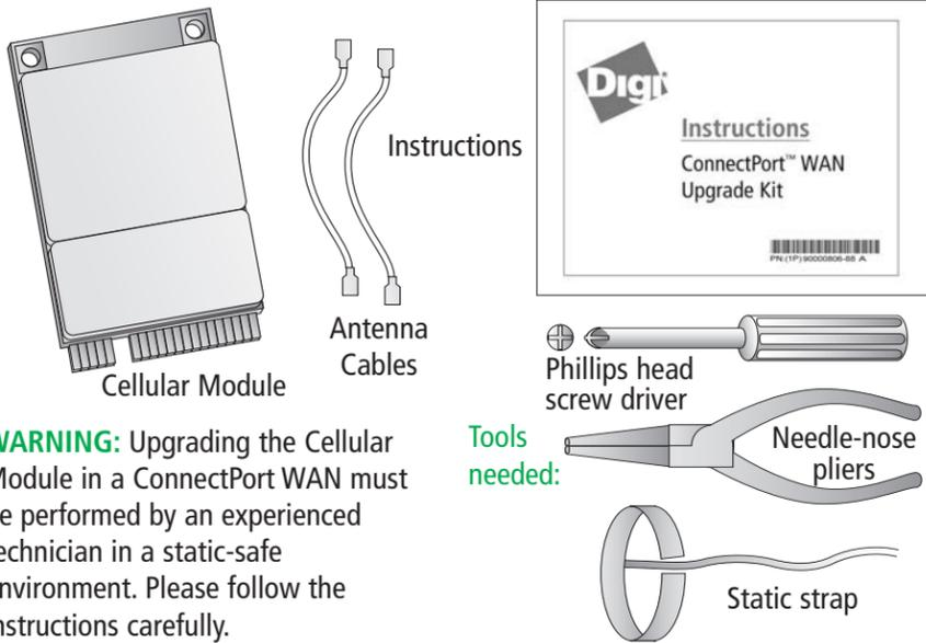
**WARNING:** Upgrading the Cellular Module in a ConnectPort WAN must be performed by an experienced technician in a static-safe environment. Please follow the instructions carefully.
