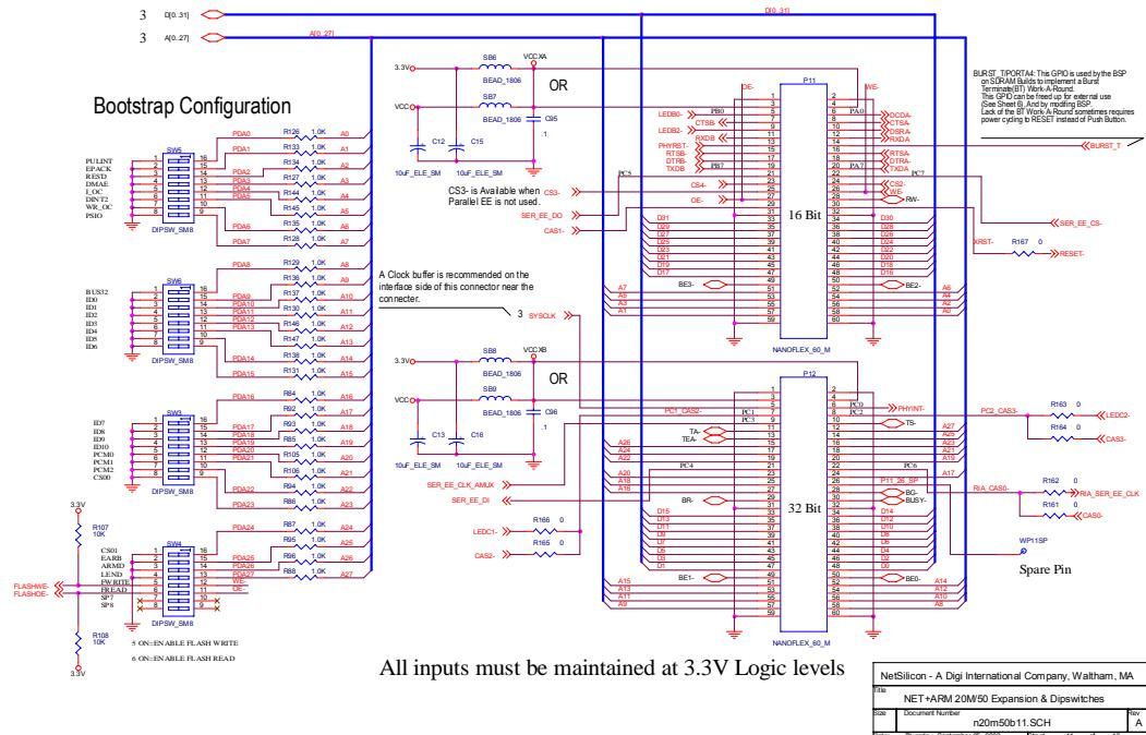
All inputs must be maintained at 3.3V Logic levels
