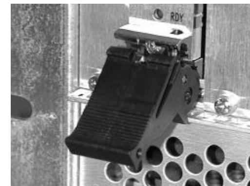
Figure 1. Ejector Handle in Unlocked Position
