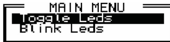
Using the keypad, the operator can move the highlight with the **UP/DOWN** arrow keys. Press the **ENTER** key to select the highlighted item.
