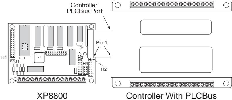
Figure 14-2. Connecting XP8800 Expansion Board to Controller PLCBus
