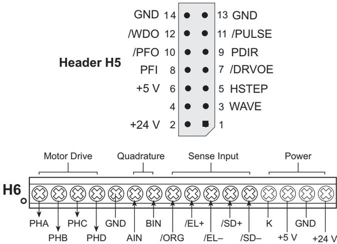
Figure 15-1. XP8800 Output Header H5 and Terminal Block H6
