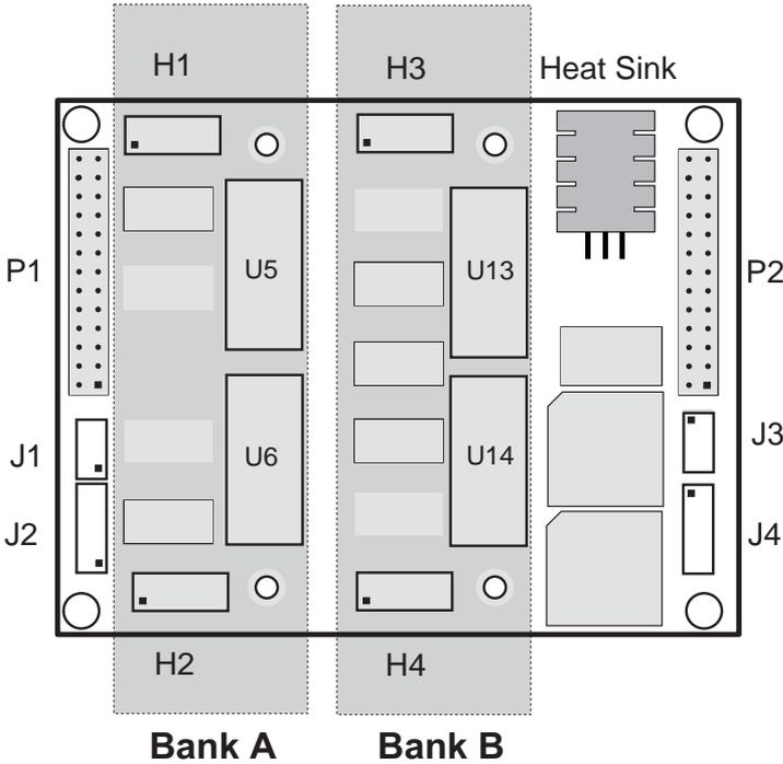
**Figure 3-1. Outline of Input/Output Banks A and B**
