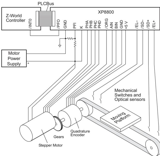
Figure 15-2. Sample Stepper Motor Connection to XP8800
