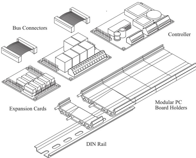
**Figure C-3. Mounting Expansion Boards on DIN Rail**
