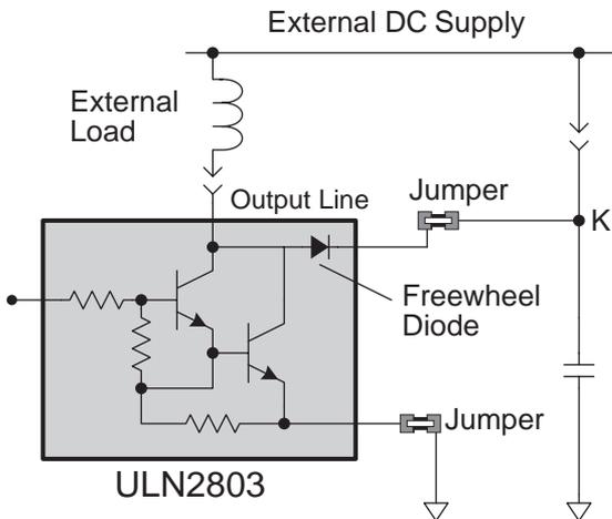
**Figure 3-5. XP8100 Series Sinking Driver Output**
