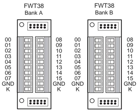
Figure 4-4. FWT38 Pinouts
