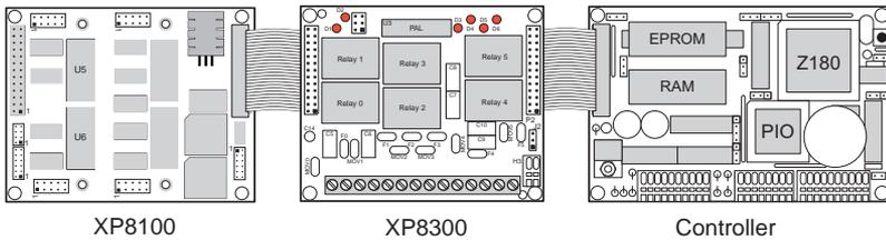
**Figure B-1. Connecting Multiple Expansion Boards**
