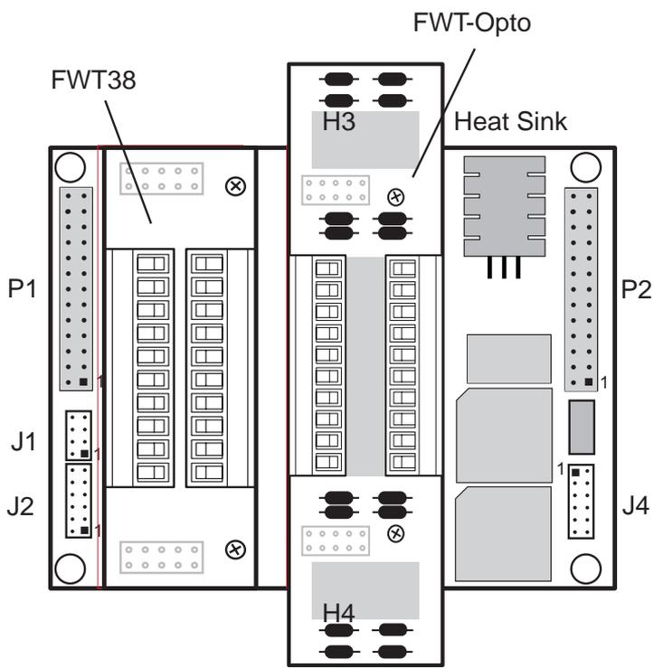
Figure 4-1. Top View of XP8100 with FWT Modules
