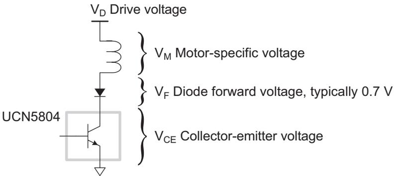
**Figure 15-9. Voltage Drops Associated with UCN5804 Motor Driver Chip**
