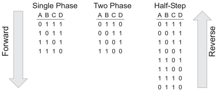
**Figure 15-7. Illustration of Phase Signals A, B, C, and D Produced by Motor Driver Chip**
