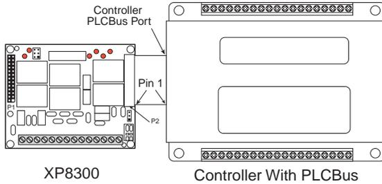
**Figure 7-1. Connecting XP8300 Expansion Board to Controller PLCBus**
