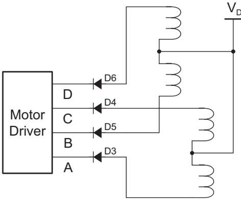
**Figure 15-8. Connection of Phase Lines to Motor**
