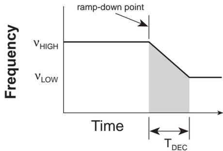
Figure 15-6. Calculating the Number of Pulses
