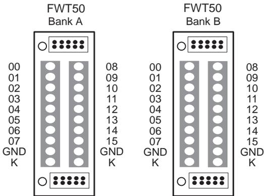
Figure 4-6. FWT50 Pinouts
