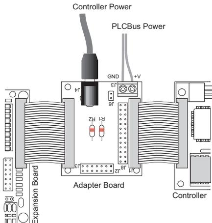
**Figure C-3. Adapter Board Connections**
