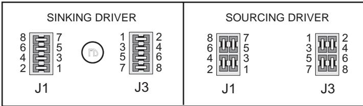
**Figure 3-4. Jumper Configurations for Sinking and Sourcing Outputs**
