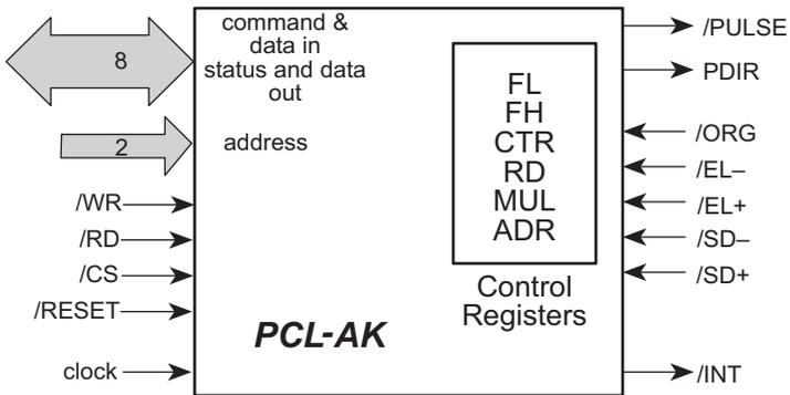
**Figure 15-5. Block Diagram of PCL-AK Pulse Generator Chip**
