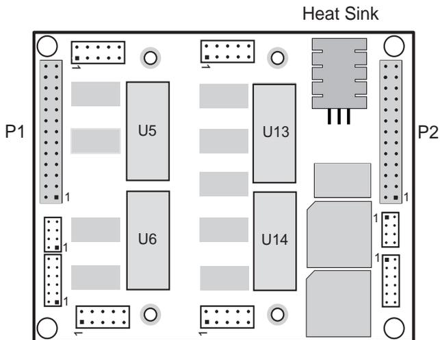
**Figure 3-7. U5, U6, U13 and U14 Locations of Sinking Drivers**
