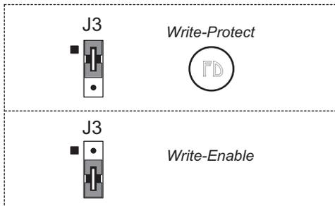
Figure 11-6. XP8500 EEPROM Jumper Settings for Header J3
