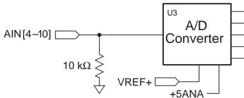
**Figure 11-7. Schematic of XP8500 Unconditioned Inputs**
