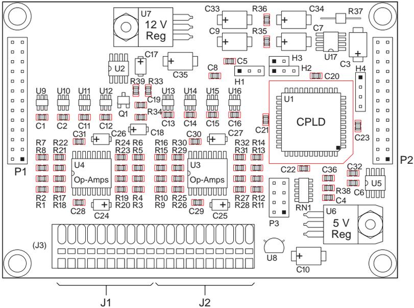
Figure 18-1. XP8900 Series Board Layout
