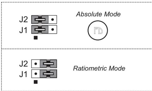
Figure 11-2. XP8500 Jumper Settings for Absolute or Ratiometric Modes
