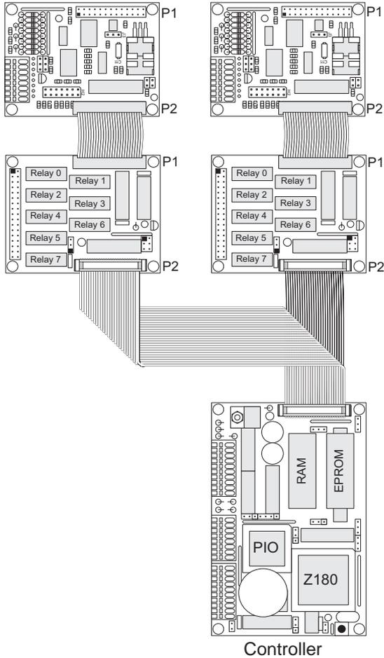
**Figure B-2. Use of Y Cable to Connect Multiple Expansion Boards**
