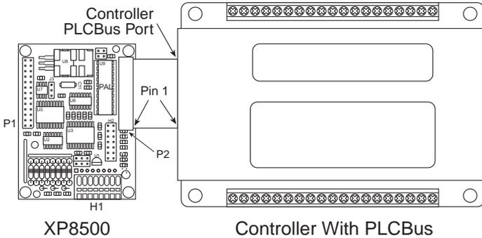
**Figure 10-2. Connecting XP8500 Expansion Board to Controller PLCBus**
