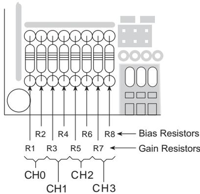
**Figure 11-4. Location of XP8500 Gain and Bias Resistors**
