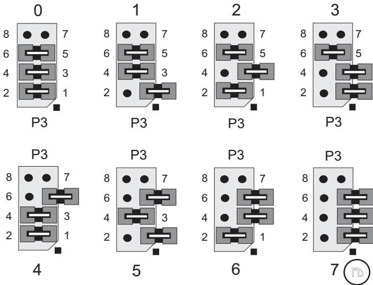
**Figure 18-3. P3 Jumper Settings for XP8900 Series PLCBus Addresses**
