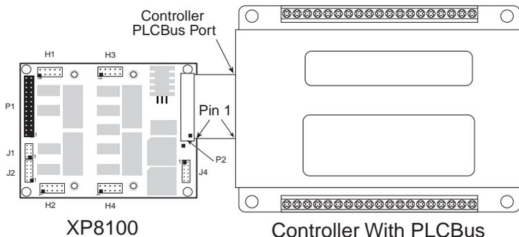
**Figure 2-2. Connecting XP8100 Expansion Board to Controller PLCBus**
