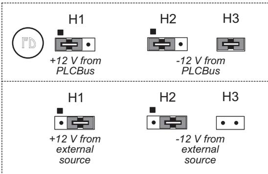
**Figure 19-2. XP8900 Series  $\pm 12$  V Supply Jumper Settings**
