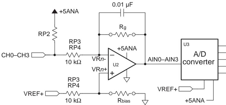
Figure 11-3. Schematic of XP8500 Signal Conditioning
