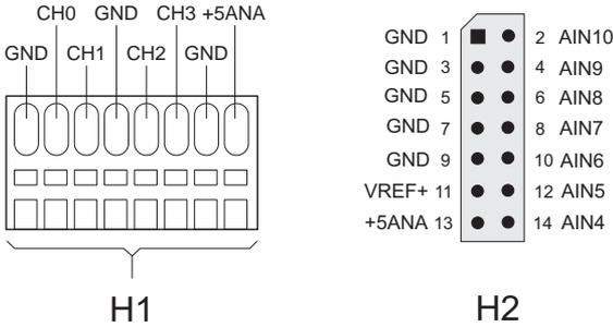
Figure 11-1. XP8500 Pin Assignments
