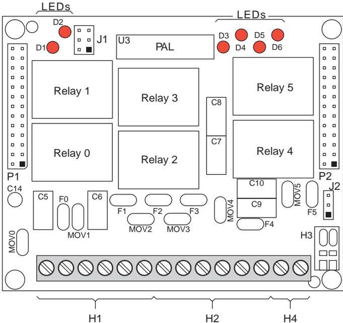
**Figure 6-2. XP8300 Relay Expansion Board Layout**
