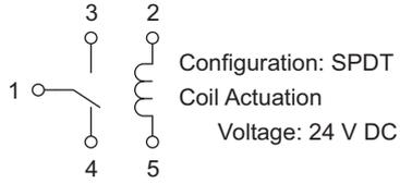
Figure 7-2. Relay Circuit
