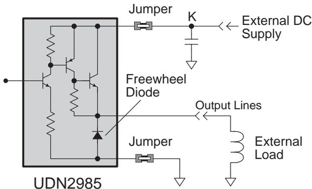
**Figure 3-6. XP8100 Series Sourcing Driver Output**
