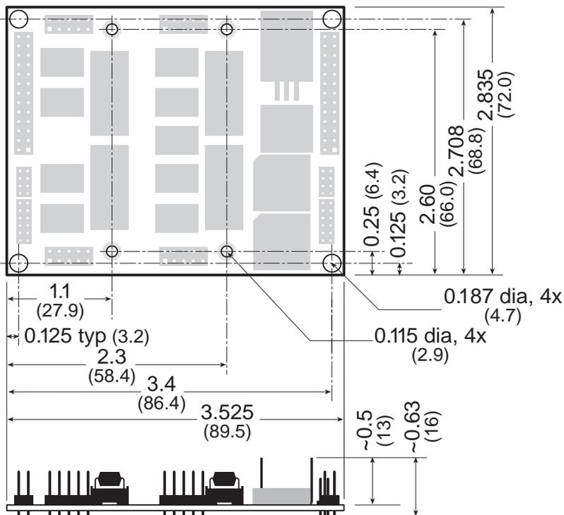
**Figure 1-6. XP8100 Series Board Dimensions**
