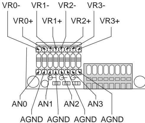
Figure 11-10. XP8500 LMC660 Op-Amp Test Points
