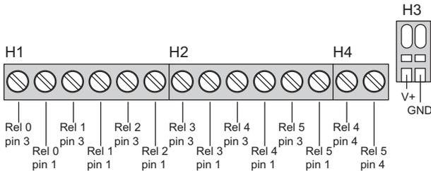
Figure 7-3. Relay Connection Pins
