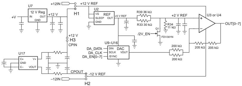
**Figure 19-3. Schematic Illustration of D/A Conversion in XP8900 Series**
