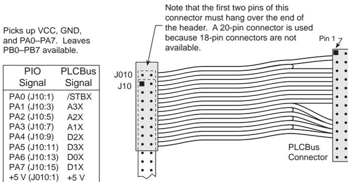
**Figure C-2. BL1100 Expander Cable Connection**
