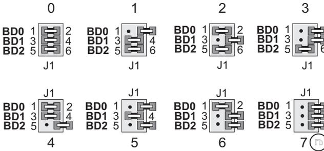
**Figure 7-4. J1 Jumper Settings for XP8300 Board PLCBus Addresses**
