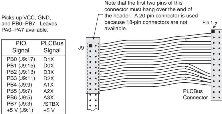
**Figure C-1. BL1000 Expander Cable Connection**
