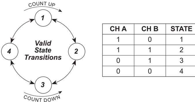
**Figure 15-11. HCTL-2016 Quadrature Counting Operation**
