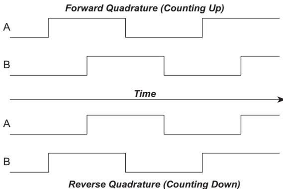
**Figure 15-10. HCTL-2016 Quadrature Counting Operation**
