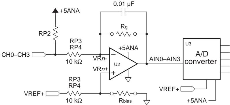
Figure 11-8. Schematic of XP8500 Signal Conditioning
