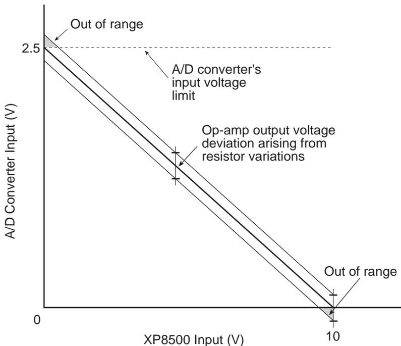
**Figure 11-9. Effects on A/D Converter Input from Adjusting Resistor Values**
