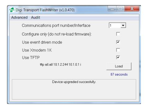
This means the WR41V1 has been successfully flashed and correct communication with the internal radio module (if fitted) verified.
