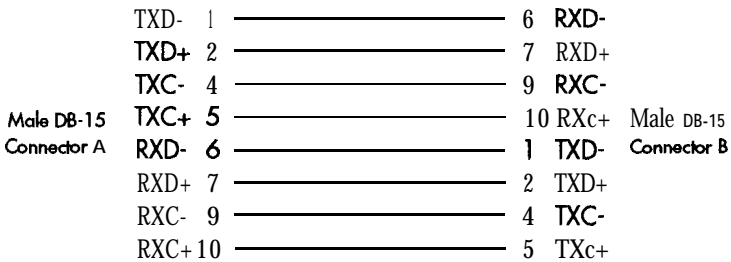
Figure 18, Loopback cable diagram
