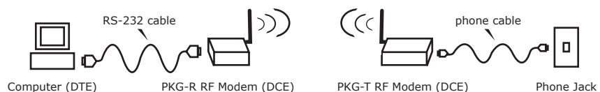
Figure 9. RF Link Configuration Method Setup
