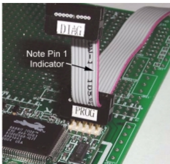
Figure 6. Connect Programming Cable to RCM2300
