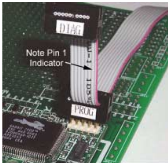
Figure 5. Connect Programming Cable to RCM2200
