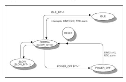
RTC alarm could not be used, because instead of the internal RTC, an external one is used.
