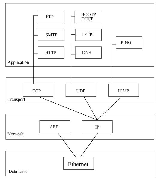
Figure 5.1 TCP/IP Protocol Flow
