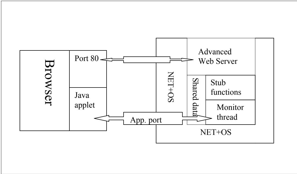
On the left side of the diagram is a browser. This could be MS Internet Explorer, Mozilla firefox or Netscape Navigator. For that matter it could be any browser that supports java applets. The three that I mentioned are the “big three”. The block marked port 80 represents standard web pages that would be using the browser for communicating with the advanced web server. I call it port 80 because the standard port for communicating with web servers is port 80.
