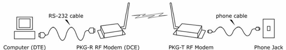
Figure 3-02. Hardware Setup - Wireless Link Method
