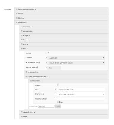
Open the configuration profile for the 63xx-series router and make the following changes.
