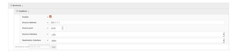
When the device is configured, the source devices that request to get access to the multicast will receive the data stream from the destination device.
