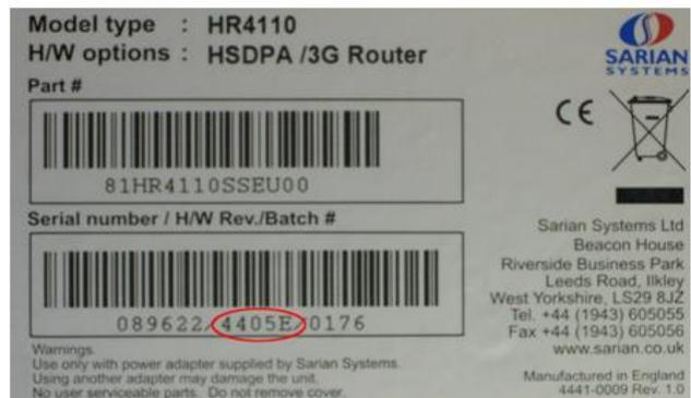
Above are the two label types, the red ellipses highlight where the hardware revisions are located. The table 1 (at the end of this document) details the hardware revision and the corresponding hardware and firmware configuration.
