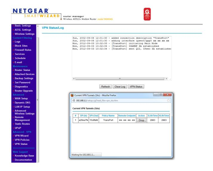
From the menu on the left choose Diagnostics, enter the IP address of a device on the remote LAN, tick "Ping VPN" then click Ping:
