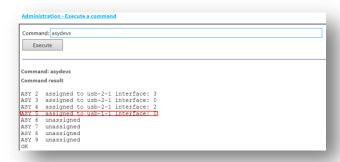
In this example, the GPS module has **ASY 5** assigned.
