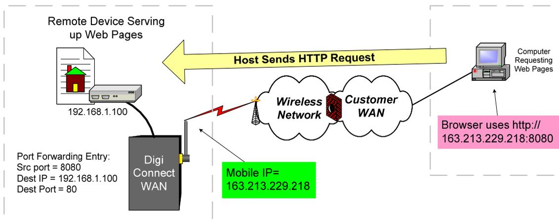
The device's HTTP server uses the default TCP port 80. The Digi cellular gateway also uses TCP port 80 for its built-in web server. To avoid conflicts there are two methods:
