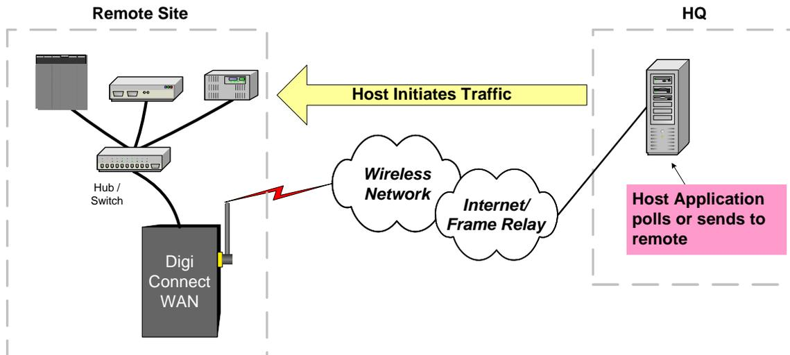
**Theory of Operation:** Communications applications such as SCADA polling, remote printing, or other host-initiated traffic can be sent over the cellular network to the remote device or devices via the Digi cellular gateway. The Digi cellular gateway forwards IP traffic destined for a specific port or port range on the cellular interface, to a private IP address on the Ethernet "side" of the Digi cellular gateway.
