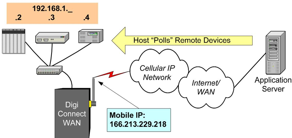
Note the devices can still use the default Modbus/TCP port number of 502 since the Digi cellular gateway's port forwarding can use different source and destination port numbers.
