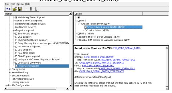
Select Digi Connect ME 9210 on Devboard in the Linux Kernel Configuration System Type. Enable Serial port A with RX/TX only (CONFIG\_CME9210JS\_SERIAL\_PORTA\_RXTX):
