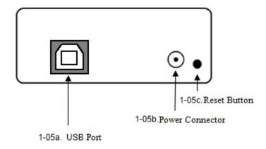
To facilitate ease of use, the RS-232 and RS-485 variants of the XBee-PRO XSC RF Modem include a mini-USB port for configuration of the radio as shown below:
