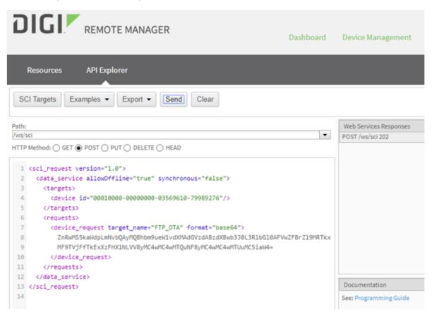
The next time the Connect Sensor is scheduled to connect to Remote Manager, it will start the modern firmware update process. To cause the device to connect immediately, press the Wake button on the device.
