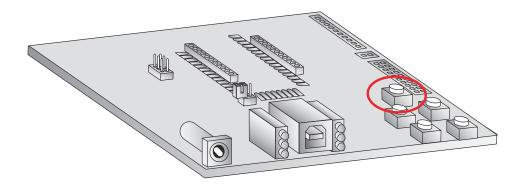
Pressing this button resets the module, but will not clear any changes written to the module. Pressing this button will also reset the COM port for the board.
