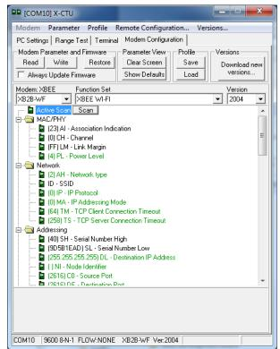
5. The XBee will then scan for available access points and routers in the area and bring up the **Scan** window, shown below:
