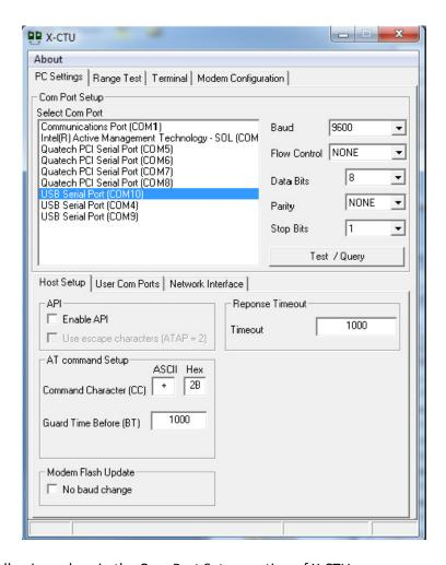
2. Set the following values in the Com Port Setup section of X-CTU:
