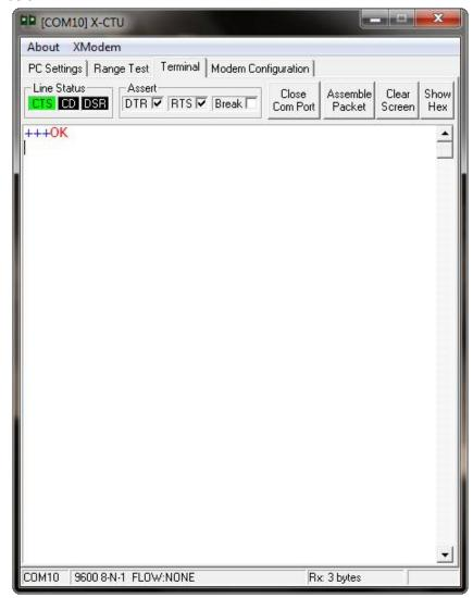
3. Type atsm1 and press the Enter key to enable the deep sleep mode.
