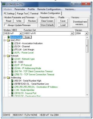
4. To find the available access points and routers within the module's range, scroll to the top of the settings list and click on **Active Scan**. Then click on the **Scan** button that will appear.
