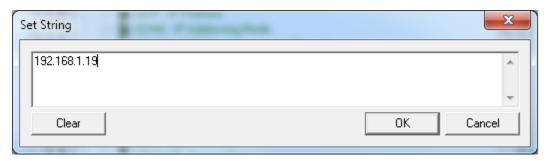
13. Enter the **Module IP Address** from module 2 into module 1's **Destination IP Address**, and the **Module IP Address** for module 1 into module 2's **Destination IP Address**.
