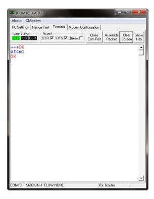
5. To exit sleep mode, wake the module up by checking the **DTR** box. The CTS light will come back on and the XBee Wi-Fi module will wake up.
