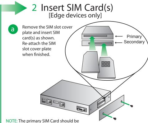
installed in the upper SIM slot, and the contacts should be face down. In the lower slot, the contacts should be face up. In both cases, the end of the SIM card with the chamfered corner should be inserted first.
