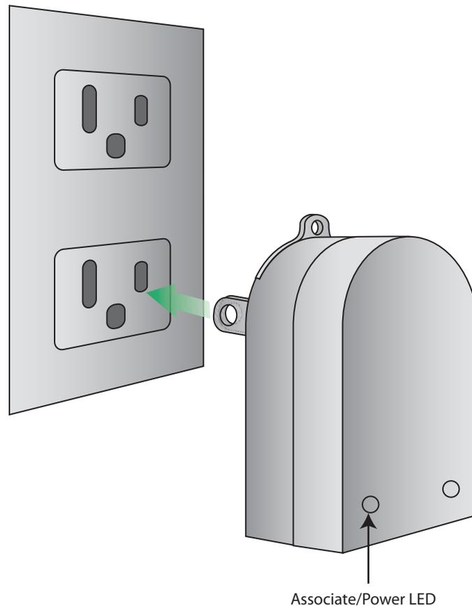
2. Observe the Associate/Power LED. When it changes from solid green to blinking green, the XBee Wall Router has joined the ZigBee network.
