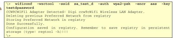
This command creates a connection like the one seen in topic 11.9.6.2 but, additionally, this entry is added to the Registry:
