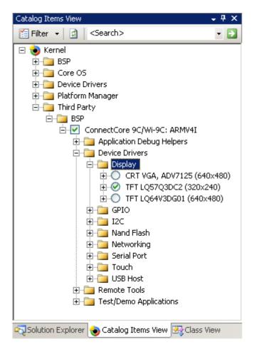
The catalog allows the choice of a VGA or TFT driver.
