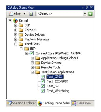
The **Test\_GPIO** is a C# application that assigns **GPIO48** and **GPIO49** to **LED1** and **LED2** respectively, and **GPIO72** and **GPIO69** to **BUTTON1** and **BUTTON2** respectively. The GPIOs assigned to LEDs are configured as outputs and the ones assigned to buttons are configured as inputs.
