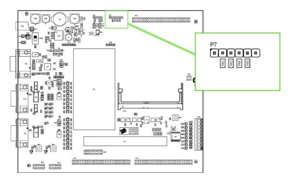
This test transmits and receives data using the same port. For this purpose, the lines **SPI\_DOUT** and **SPI\_DIN** of the SPI port must be interconnected. In the development board, these port B lines are accessible in connector **P7**, pins 2 and 3.
