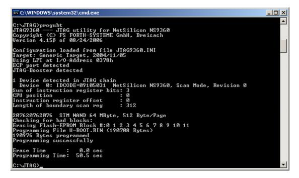
The programming takes approximately 60 seconds, after which the message **Programming successfully** is displayed.
