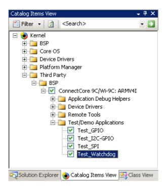
**Test\_WatchDog** is a C# multi-thread application that uses some functions to handle and refresh a watchdog timer.
