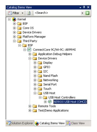
The USB host (OHCI) driver supports only the interface. Specific USB devices are supported by USB class drivers, like Human Input Devices (HID) class driver (for mice and keyboards), the Storage class driver (for USB flash disks), and so on.
