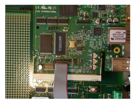
2. Connect the adapter cable to the hardware module plugged into the development board.
