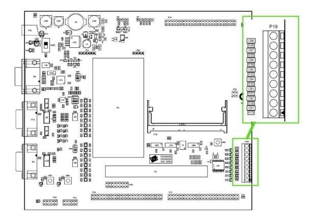
To change the status of an output, click the switch drawing in the **Test\_I2C-GPIO** application. To change the value of an input, force it by hardware to ground (0V) or to Vcc (5V).
