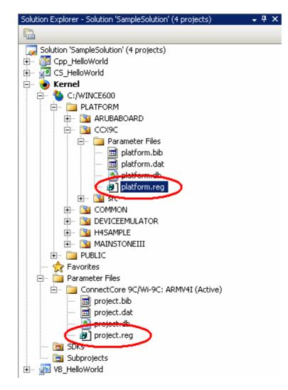
For example, some Registry information has been included for the FTP and the TELNET servers in **Platform.reg**. Double-click it to access the Registry information. Then expand **HKEY\_LOCAL\_MACHINE > Comm** and select **FTPD** and **TELNETD**.
