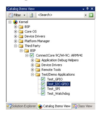
The **Test\_I2C-GPIO** is a C# application that works with some of the  $I^2C$  registers (input port, output port and configuration). It is in the **Windows\** folder.
