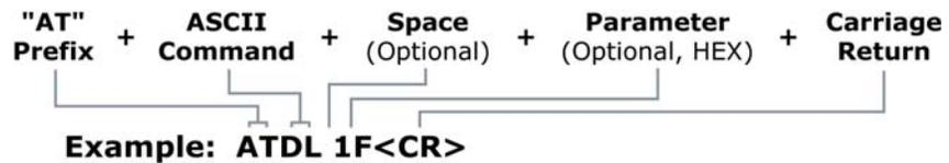
NOTE: To read a parameter value stored in a register, leave the parameter field blank.
