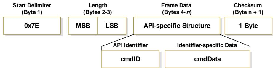
The cmdID frame (API-identifier) indicates which API messages will be contained in the cmdData frame (Identifier-specific data). Refer to the sections that follow for more information regarding the supported API types. Note that multi-byte values are sent big endian.
