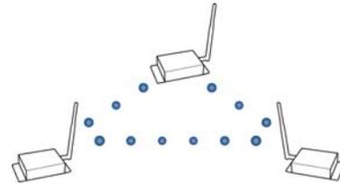
A peer-to-peer network can be established by configuring each modem to operate as an End Device (CE = 0), disabling End Device Association on all modems (A1 = 0) and setting ID and CH parameters to be identical across the network.
