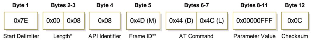
\* Length [Bytes] = API Identifier + Frame ID + AT Command + Parameter Value
