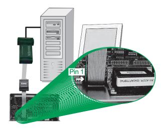
Connect ribbon cable from Raven to JTAG header on development board
