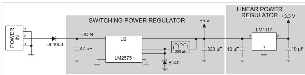
**Figure 11. Power Supply Circuit Used on Prototyping Boards**
