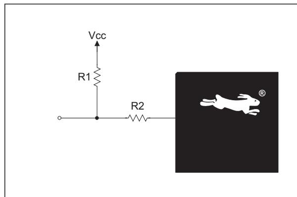
**Figure 1. Pulled-Up Input**
