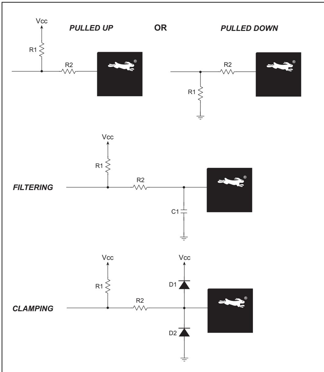
**Figure 9. Digital Input Setup**
