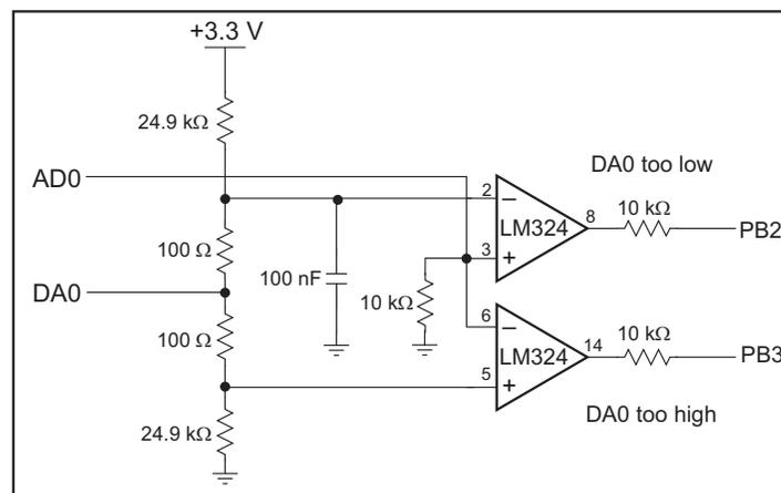
Figure 6. Discrete Inexpensive Op-Amp Based A/D Converter
