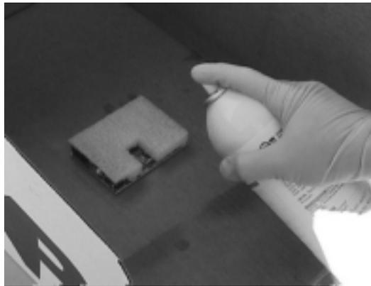
**Figure 5. Applying Coating to Masked Board**
