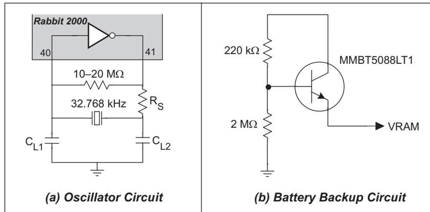
**Figure 1. High-Impedance Circuits Recommended for Conformal Coating**
