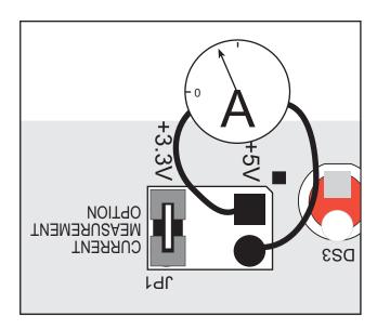
Figure B-5. Prototyping Board Current-Measurement Option
