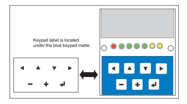
Figure C-5. Removing and Inserting Keypad Label
