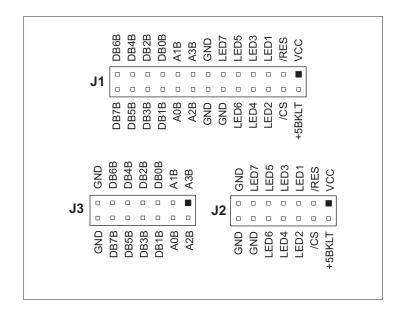
Figure C-6. LCD/Keypad Module Pinouts
