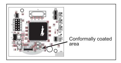
Figure A-5. RCM3100 Areas Receiving Conformal Coating
