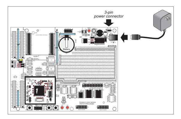
Figure 3. Power Supply Connections
