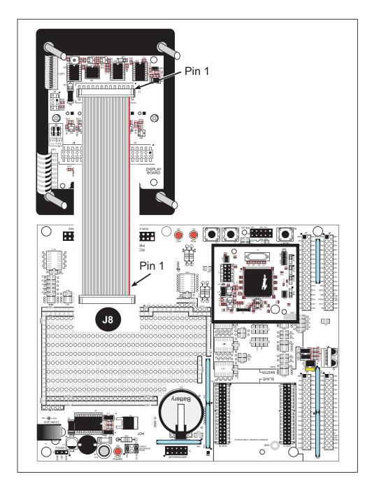
Figure C-10. Connecting LCD/Keypad Module to RCM30/31/32XX Prototyping Board
