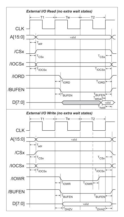
Figure A-4. External I/O Read and Write Cycles—No Extra Wait States
