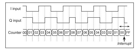
Figure E-2. Operation of Quadrature Decoder Counter
