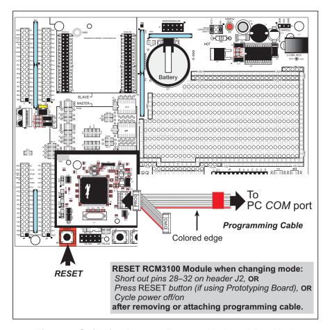
Figure 7. Switching Between Program Mode and Run Mode
