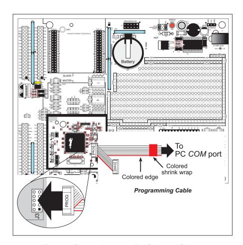
Figure 2. Connect Programming Cable to RCM3100
