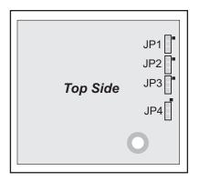
Figure A-6. Location of RCM3100 Configurable Positions
