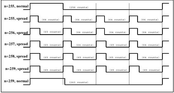
Figure E-1. PWM Outputs for Various Normal and Spread Modes
