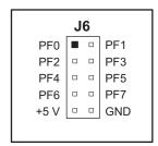
Figure B-6. Prototyping Board Motor Encoder Connector Pinout
