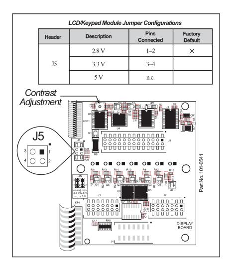
Figure C-3. LCD/Keypad Module Voltage Settings
