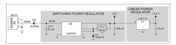
Figure B-3. Prototyping Board Power Supply
