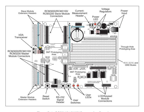
Figure B-1. RCM30/31/32XX Prototyping Board
