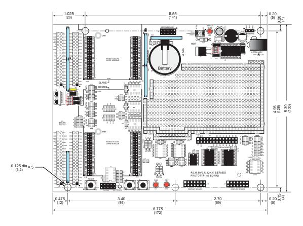
Figure B-2. RCM30/31/32XX Prototyping Board Dimensions
