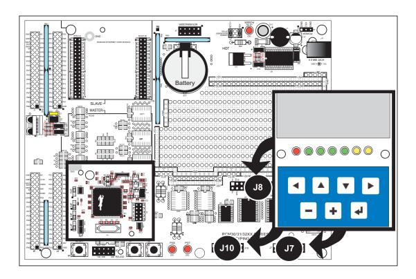
Figure C-7. Install LCD/Keypad Module on Prototyping Board
