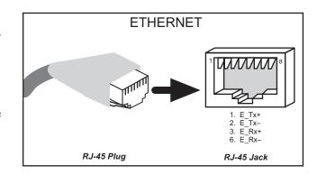
Figure 7. RJ-45 Ethernet Port Pinout
