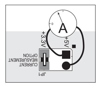
Figure B-5. Prototyping Board Current-Measurement Option
