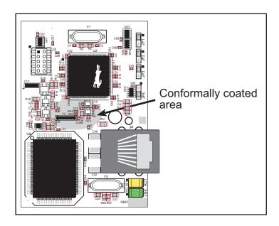
Figure A-5. RCM3000 Areas Receiving Conformal Coating
