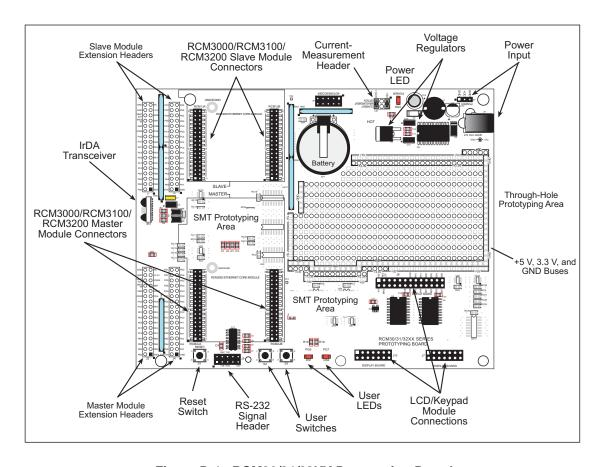
Figure B-1. RCM30/31/32XX Prototyping Board
