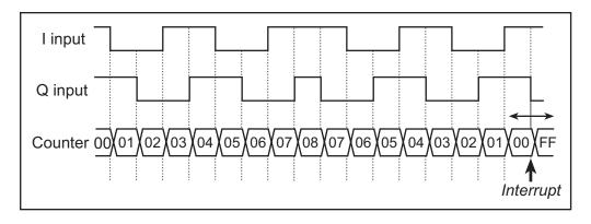
Figure E-2. Operation of Quadrature Decoder Counter
