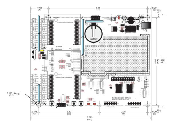
Figure B-2. RCM30/31/32XX Prototyping Board Dimensions
