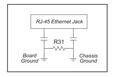
Figure 8. Isolation Resistor R31
