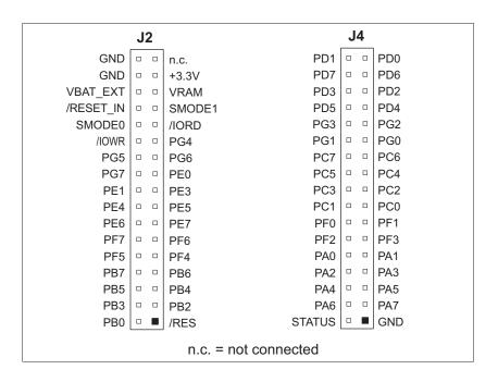
Figure B-4. RCM30/31/32XX Prototyping Board Pinout (Top View)
