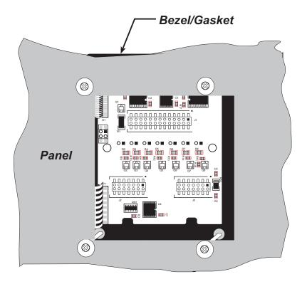
Figure C-9. LCD/Keypad Module Mounted in Panel (rear view)
