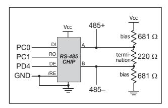
The diagram shows the connections. You will have to connect PC0 and PC1 (Serial Port D) on the RCM30/31/32XX Prototyping Board to the RS-485 transceiver, and you will connect PD4 to the RS-485 transceiver to enable or disable the RS-485 transmitter.
