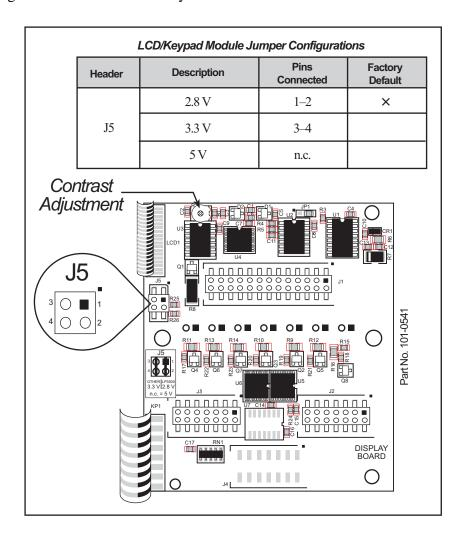
Figure C-3. LCD/Keypad Module Voltage Settings
