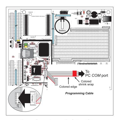
Figure 2. Connect Programming Cable to RCM3000
