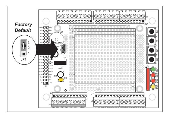
Figure C-4. Demonstration Board Header JP1 (Buzzer On/Off)
