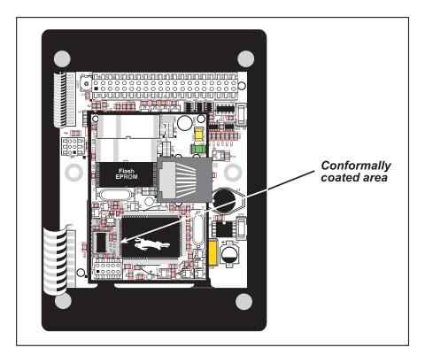
Figure A-3. OP6800 Areas Receiving Conformal Coating
