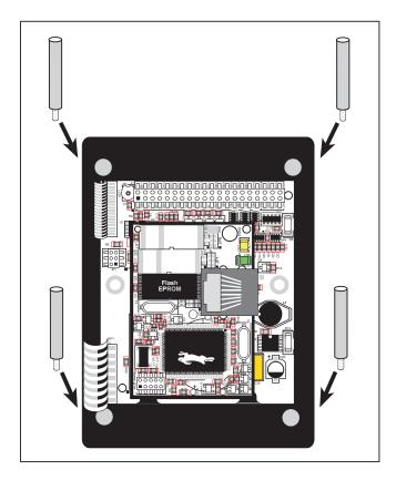
Figure 2. Screw In Standoffs Into OP6800 Mounting Threads
