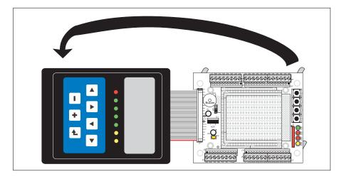
Figure C-6. Mounting Demonstration Board on OP6800
