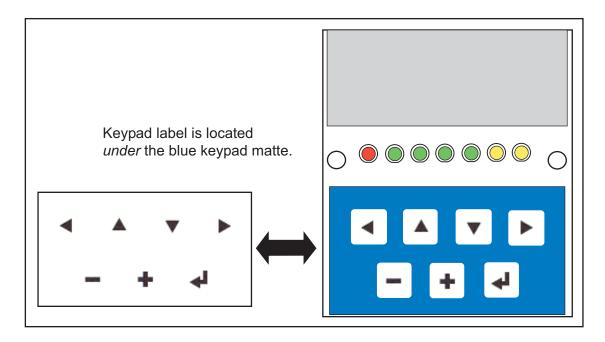
Figure 18. Removing and Inserting Keypad Label
