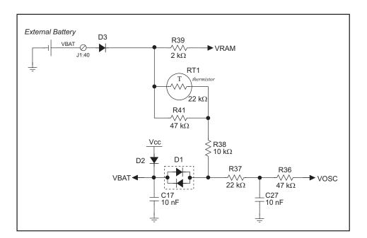
Figure B-1 shows the battery-backup circuit located on the OP6800 module.
