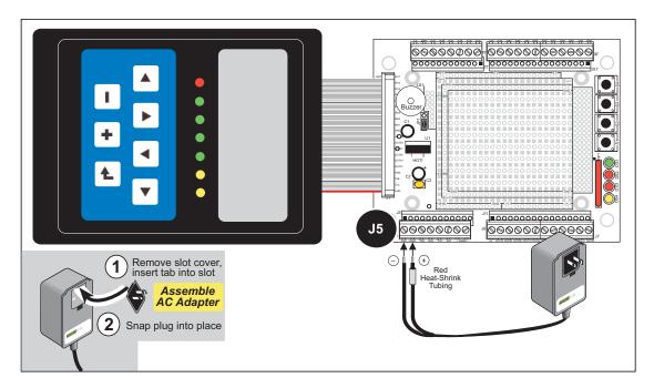
Figure 4. Power Supply Connections
