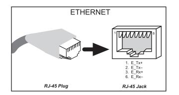
Figure 13. RJ-45 Ethernet Port Pinout
