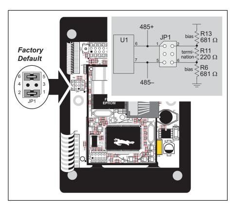
Figure 12. RS-485 Termination and Bias Resistors
