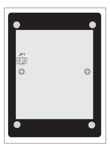
Figure A-4. Location of BL2100 Configurable Positions
