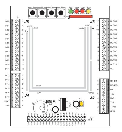
Figure C-5. OP6800 Demonstration Board Pinout
