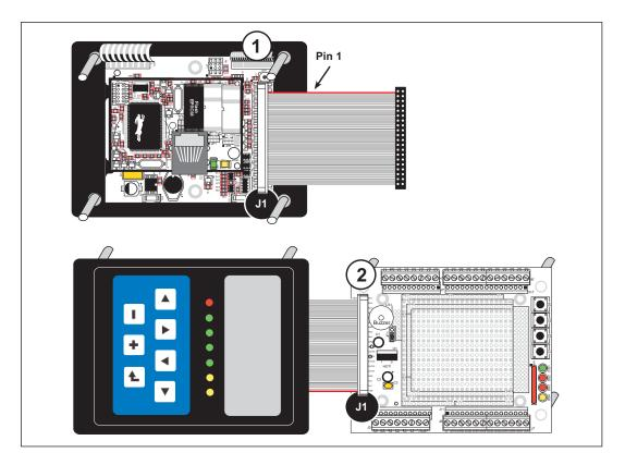
Figure 3. Connect the OP6800 to the Demonstration Board
