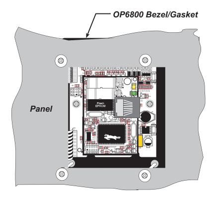
Figure 21. OP6800 Mounted in Panel (rear view)
