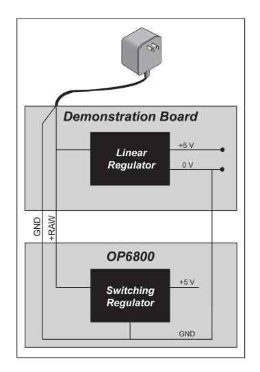
Figure C-2. Power Distribution to OP6800 and Demonstration Board
