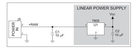
Figure C-3. Demonstration Board Power Supply
