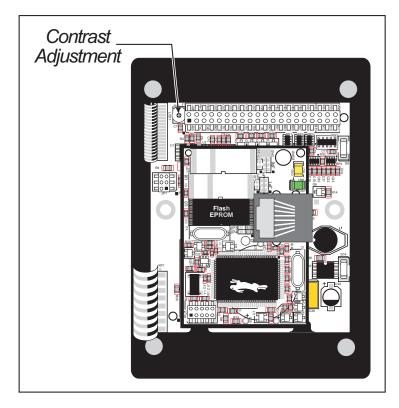
Figure 5. LCD Contrast Adjustment
