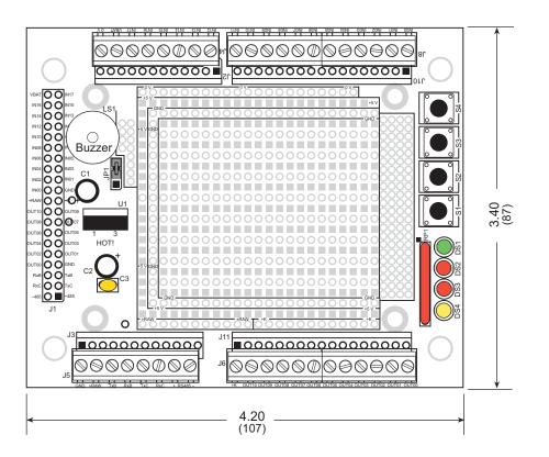
Figure C-1. OP6800 Demonstration Board Dimensions
