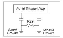
Figure 14. Isolation Resistor R29
