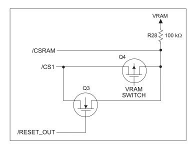
Figure B-1. Chip Select Circuit
