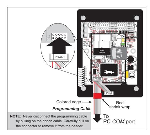
Figure 6. Programming Cable Connections
