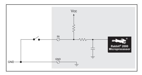
Figure 9. OP6800 Digital Inputs
