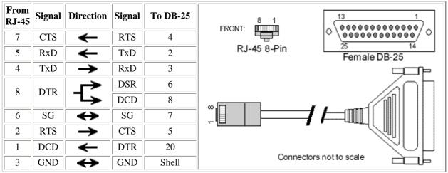
\* Arrows indicate which direction the signal is flowing
